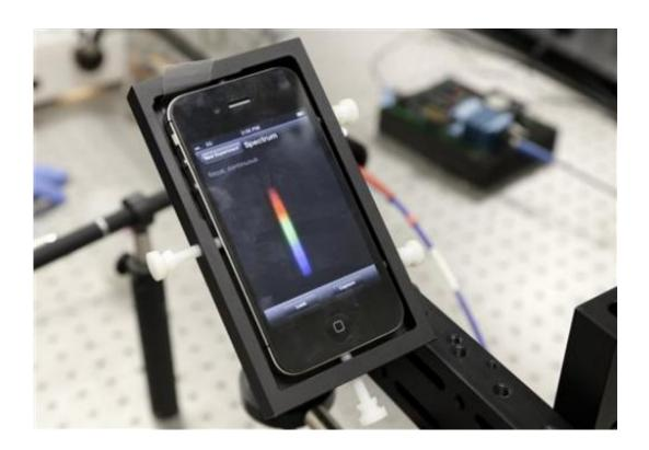
A handheld biosensor was developed by researchers at the University of Illinois, Urbana-Champaign, is shown June 21, 2013 in Urbana, Ill. Thanks to a cradle and app that turn your smartphone into a handheld biosensor, you may soon be able to run on-the-spot tests for food safety, environmental toxins, medical diagnostics and more. (AP Photo/Michael Conroy)
