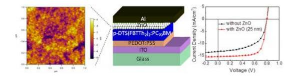
(Left) A ZnO optical spacer viewed under an atomic force microscope. (Center) The device structure of the small-molecule solar cell. (Right) Solar cell performance with and without an optical spacer. Credit: Aung Ko Ko Kyaw, et al. ©2013 American Chemical Society
