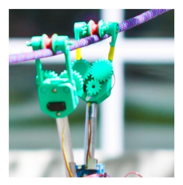
SkySweeper is V-shaped with a motor-driven "elbow" and its ends are equipped with clamps that open and close as necessary to move it down utility lines, searching for damage, inch by inch. It was designed by graduate student Nick Morozovsky in the Coordinated Robotics Lab led by mechanical and aerospace engineering professor Tom Bewley. Credit: UC San Diego Jacobs School of Engineering.
