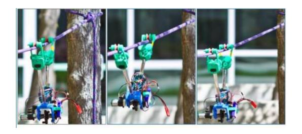
SkySweeper is V-shaped with a motor-driven "elbow" and its ends are equipped with clamps that open and close as necessary to move it down utility lines, searching for damage, inch by inch. It was designed by graduate student Nick Morozovsky in the Coordinated Robotics Lab led by mechanical and aerospace engineering professor Tom Bewley. Credit: UC San Diego Jacobs School of Engineering.
