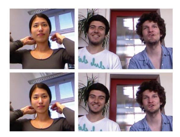
Innovative software rotates the face of the person on screen during video conferences in order to make eye contact. Credit: Computer Graphics Laboratory / ETH Zurich
