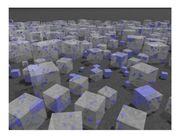
Palladium nanocubes interacting with hydrogen gas were directly observed through in situ luminescence to reveal that size can make a much bigger difference on phase transformations than scientists previously believed. Credit: Berkeley Lab
