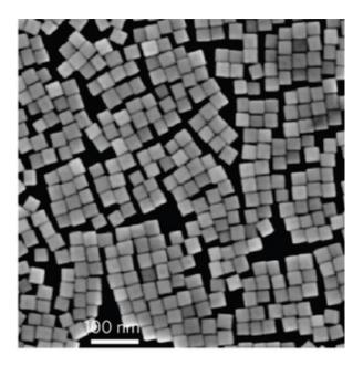
This scanning electron micrograph shows palladium nanocubes with a side length of approximately 32 nanometers. Credit: Berkeley Lab
