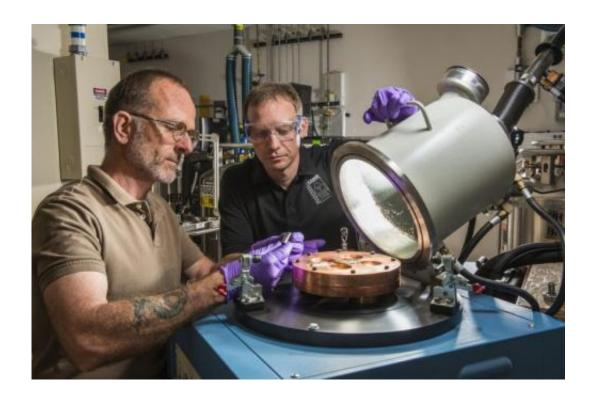
Sandia National Laboratories' Mark Reece, left, and Don Susan examine a new shape memory alloy button they have removed from an arc-melter. Several new alloys have been developed at Sandia. Credit: Randy Montoya
