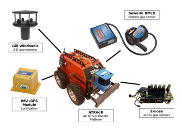
(Phys.org) —A team of researchers at Sweden's AASS Research Centre at Orebro University has built a robot prototype that moves itself around in its environment searching for methane leaks. In its initial testing phase, the robot, dubbed Gasbot, was able to sniff out artificially created methane sources in a former landfill and in an underground tunnel.
