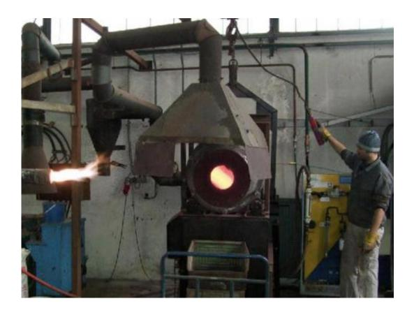
Rotary kiln: used in the thermal-chemical process to remove heavy metals and recover phosphorus from sewage sludge ash. Credit: ETH Zurich
