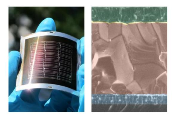
This shows the CdTe solar cells on a flexible metal foil (left) and electron microscopy (EM) image of the solar cell structure in the substrate configuration (right) with front electrical contact (uppermost layer), central CdTe layer and metal back contact (lowest layer), all deposited on the substrate (glass is used as an example for ease and clarity of EM imaging). Credit: Empa
