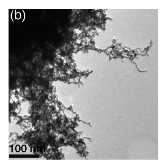
Electron microscope image of the platin/palladium aerogel (alloy ratio: 50% platine, 50% palladium). Credit: Wiley-VCH Verlag GmbH & Co. KGaA
