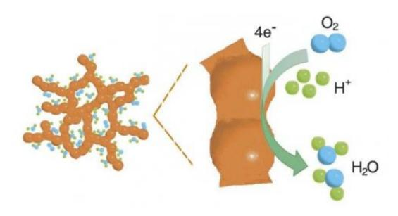
Schematic representation of the oxygen reduction reaction at the positive electrode of a low-temperature polymer electrolyte fuel cell. Each oxygen atom from the oxygen molecules fed into the cell captures two electrons, which is followed by the reaction with hydrogen nuclei to form water. Credit: Wiley-VCH Verlag GmbH & Co. KGaA
