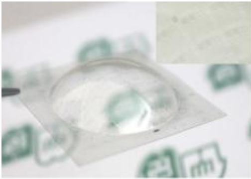
(Left) A dome-shaped all-carbon device (scale bar, 10 mm). Inset: magnified photograph (scale bar, 1 mm). (Right) Illustration of the cross-section of the air-assisted thermopressure-forming apparatus used to mold the all-carbon device. Credit: Sun, et al. ©2013 Macmillan Publishers Limited
