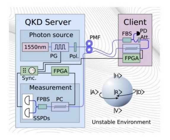
Experimental set-up for client-server rfiQKD. The server side holds a telecom wavelength (1550 nm) laser with a 1 MHz pulse generator (PG) and fixed polariser, to send light pulses to the client through a polarisation maintaining fibre (PMF). At the client side, an integrated polarisation controller (PC) encodes qubits into the polarisation of the attenuated (Att.) light. A fibre beam splitter (FBS) and photodetector (PD) continuously monitor power for malicious attacks.
