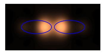
An optical antenna made of silver, represented by the two blue ellipses, can concentrate red light at a subwavelength scale. Credit: 2013 A\*STAR Institute of High Performance
