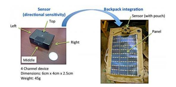
Solar sensor boxes attached to the top of mobile solar power unit packs directly measure the amount of solar irradiation (sunlight) visible to the photovoltaic panels. Credit: US Naval Research Laboratory
