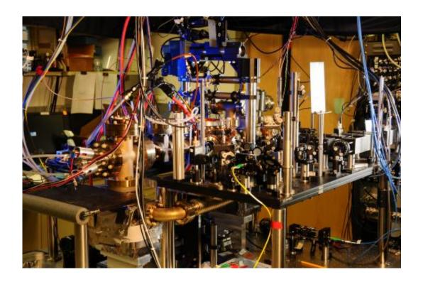
In NIST's ultra-stable ytterbium lattice atomic clock, ytterbium atoms are generated in an oven (large metal cylinder on the left) and sent to a vacuum chamber in the center of the photo to be manipulated and probed by lasers. Laser light is transported to the clock by five fibers (such as the yellow fiber in the lower center of the photo). Credit: Burrus/NIST
