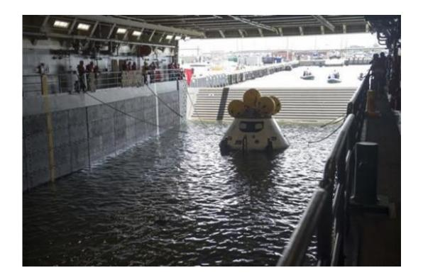
In this image provided by the U.S. Navy, sailors assigned to the amphibious transport dock ship USS Arlington practice recovering an Orion capsule Tuesday, Aug. 13, 2013 into the well deck of the USS Arlington as part of NASA's first key Orion stationary recovery test at Naval Station Norfolk. NASA is partnering with the U.S. Navy to develop procedures to recover the Orion capsule and crew after splashdown. (AP Photo/U.S. Navy, Seaman Andrew Schneider)
