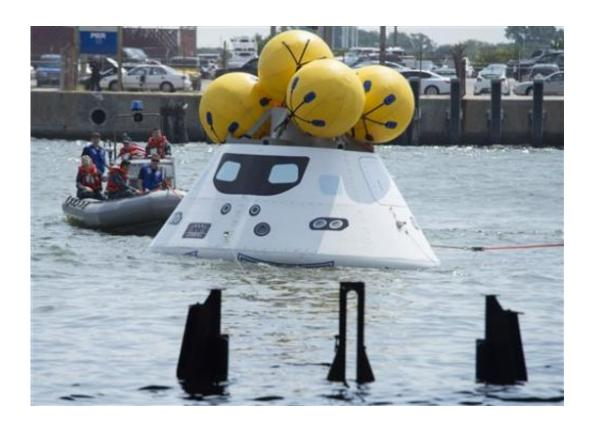
In this image provided by the U.S. Navy, sailors assigned to the amphibious transport dock ship USS Arlington practice recovering an Orion capsule Tuesday Aug. 13, 2013 into the well deck of the USS Arlington as part of NASA's first key Orion stationary recovery test at Naval Station Norfolk. NASA is partnering with the U.S. Navy to develop procedures to recover the Orion capsule and crew after splashdown. (AP Photo/U.S. Navy, Seaman Andrew Schneider)
