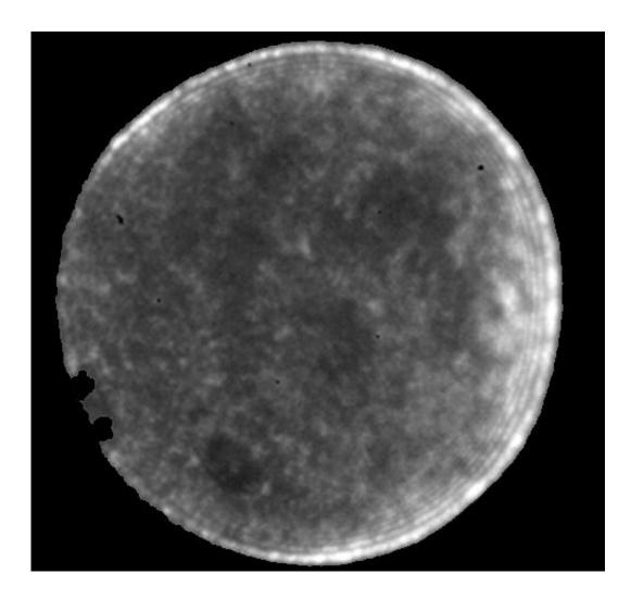
A micrograph of the nanosensor array. The florescence of each carbon nanotube changes in intensity upon binding to a target molecule. Credit: COURTESY OF THE RESEARCHERS
