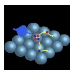
Linked quantum dots - In the new nanomaterial two or more electrons jump across the band gap as a consequence of just a single light particle (arrow with waves) being absorbed. Using special molecules the researchers have strongly linked the nanospheres (quantum dots) as a result of which the electrons can freely move and an electrical current develops in the solar cell.
