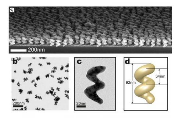
Nanostructures manufactured in parallel: Several hundred billions of helices, as well as hooks or zigzag structures, can be created with the help of vapour deposition on a pre-structured wafer (a). Ultrasonication releases the nanocomponents from the substrate so that they can be brought into colloidal suspension (b). Shape and dimensions of the structures can be controlled very exactly (c,d). Credit: Andrew G. Mark
