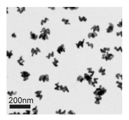
Nanohelix as a light antenna: The miniscule nanostructures can be produced very precisely and in large numbers with a new method. The colour of light they absorb can be controlled by their dimensions and composition. They are suited to filtering circularly polarised light. Credit: Andrew G. Mark
