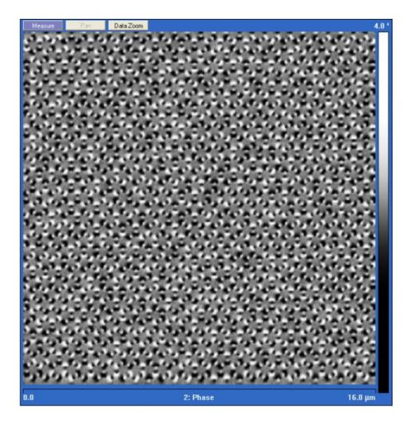
This is a magnetic force microscope image of emergent domains of ordered magnetic charges in honeycomb artificial spin ice. The black and white dots in the image are the north and south magnetic poles of the nanomagnets. Credit: Ian Gilbert, U. of I. Department of Physics and Frederick Seitz Materials Research Laboratory
