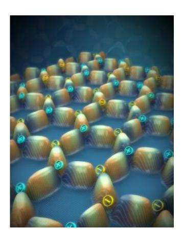
This image shows the topography of a sample of artificial kagome spin ice. The ends of the islands have been shaded blue and orange according to the magnetic polarity, and the plus and minus signs denote the net magnetic charge at each three-island vertex. Thermal annealing forms crystallites of magnetic charges of alternating sign. Credit: Alex David Jerez Roman, Ian Gilbert, and Sheng Zhang
