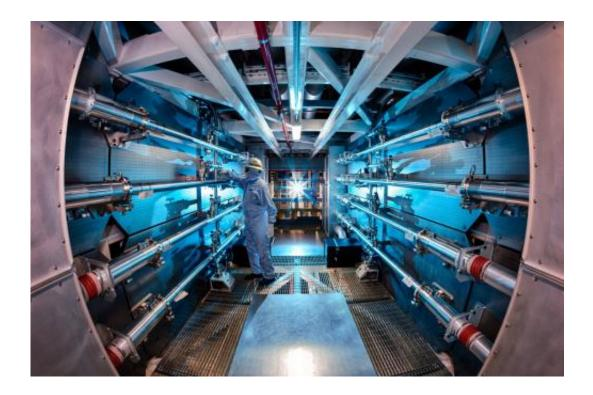
The preamplifiers of the National Ignition Facility are the first step in increasing the energy of laser beams as they make their way toward the target chamber.
