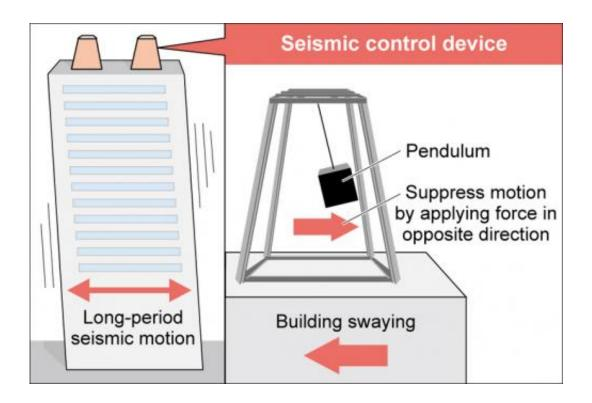
(Phys.org) —Two Japanese companies, Mitsui Fudosan and Kajima Corp, have announced plans to install quake damping pendulums atop the Shinjuku Mitsui Building in downtown Tokyo by 2015. The building, like many others in the city, was built before new quake dampening technology was developed for skyscrapers.
