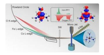
This sketch demonstrates the principle of measurement which enables to address atom-specific and state-dependent emission of photons. With the help of first principles theory the spectral features can be associated with molecular orbitals. Credit: Uni Rostock
