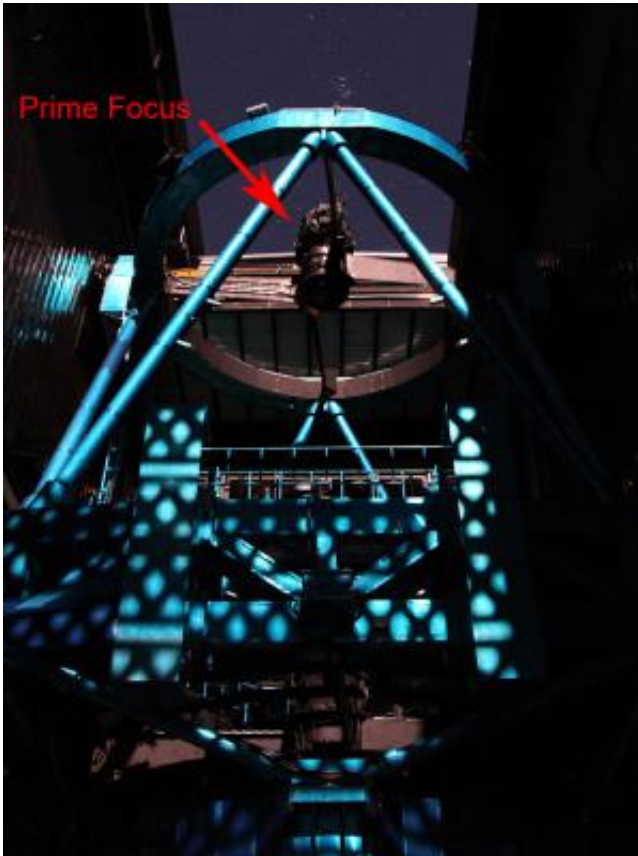
Figure 3: Views of HSC from below and above the top ring. The image on the left shows the position of HSC (without the filter exchange unit or FEU) when mounted on the inner, top ring of the Subaru Telescope. This location is at prime focus, and HSC is 15 meters above the primary mirror. (Credit: NAOJ) The
