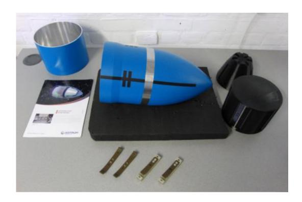
Clockwise, from top left: cylindrical section that fits to the rear of the penetrator cone (centre); the outer shell of the penetrator cone, internal payload sections; spring mechanisms to isolate payload components from outer shell and maintain the vacuum gap. Credit: ESA
