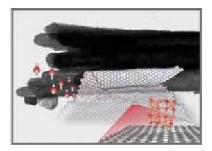
After decoration with maghemite nanoparticles the graphene spontaneously form nanoscrolls. The dark cylinders in the upper part of the image shows graphene nanoscrolls that are covered with a smooth layer of small particles. The nanoscrolls form "bundles" with 5-10 cylinders due to the interaction between the nanoscrolls. The lower part of the image show a simulated image of a graphene sheet in the scrolling process. The region zoomed show a maghemite nanoparticle attached to the graphene sheet.
