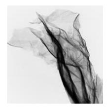
Snapshot of a partially re-opened nanoscroll. The atomic layer thick graphene resembles a thin foil with some few wrinkles.
