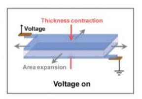
To make the speaker, a membrane of transparent, insulating rubber is sandwiched between two layers of transparent, conductive gel. The electrical connection to the power source is established outside of the active region of the device, where it does not need to be transparent. Credit: Christoph Keplinger, Jeong-Yun Sun
