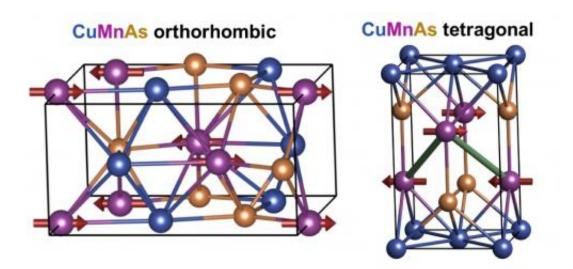
Unit cell structures of the new antiferromagnetic spintronic material, orthorhombic CuMnAs and tetragonal CuMnAs. Credit: STFC
