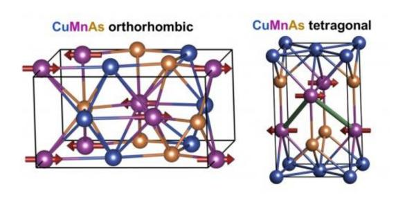
Unit cell structures of the new antiferromagnetic spintronic material, orthorhombic CuMnAs and tetragonal CuMnAs. Credit: STFC
