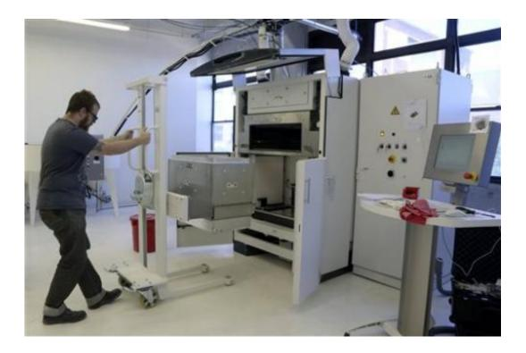
In this Wednesday, June 19, 2013 photo, an engineer at Shapeways removes finished products from a 3D Printer at the company's factory in the Queens borough of New York. Shapeways' production process is fairly simple. Anyone can upload a 3-D design to Shapeways website and submit an order to have it "printed" in plastic at the factory. The company charges based on the amount of material a design uses and then ships the final product to the customer. (AP Photo/Mary Altaffer)
