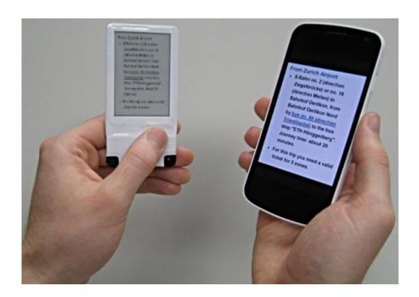
(Phys.org) —Researchers from Intel, the University of Massachusetts and the University of Washington have teamed up to build an e-paper display that can be powered by the Near Field Communication (NFC) signal from a smartphone. Called a wirelessly bistable display tag, the device works by harvesting more energy from the NFC transaction than
