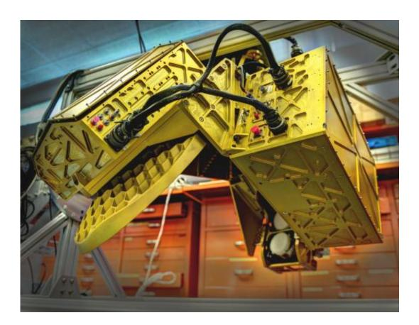
The HIWRAP dual frequency Doppler radar will hang under the Global Hawk. On the left, the golden disc is the antenna and on the right, the two small white discs are the radar beam transmitters, one for each of two frequencies. The whole apparatus spins while flying. Credit: Bill Hrybyk / NASA
