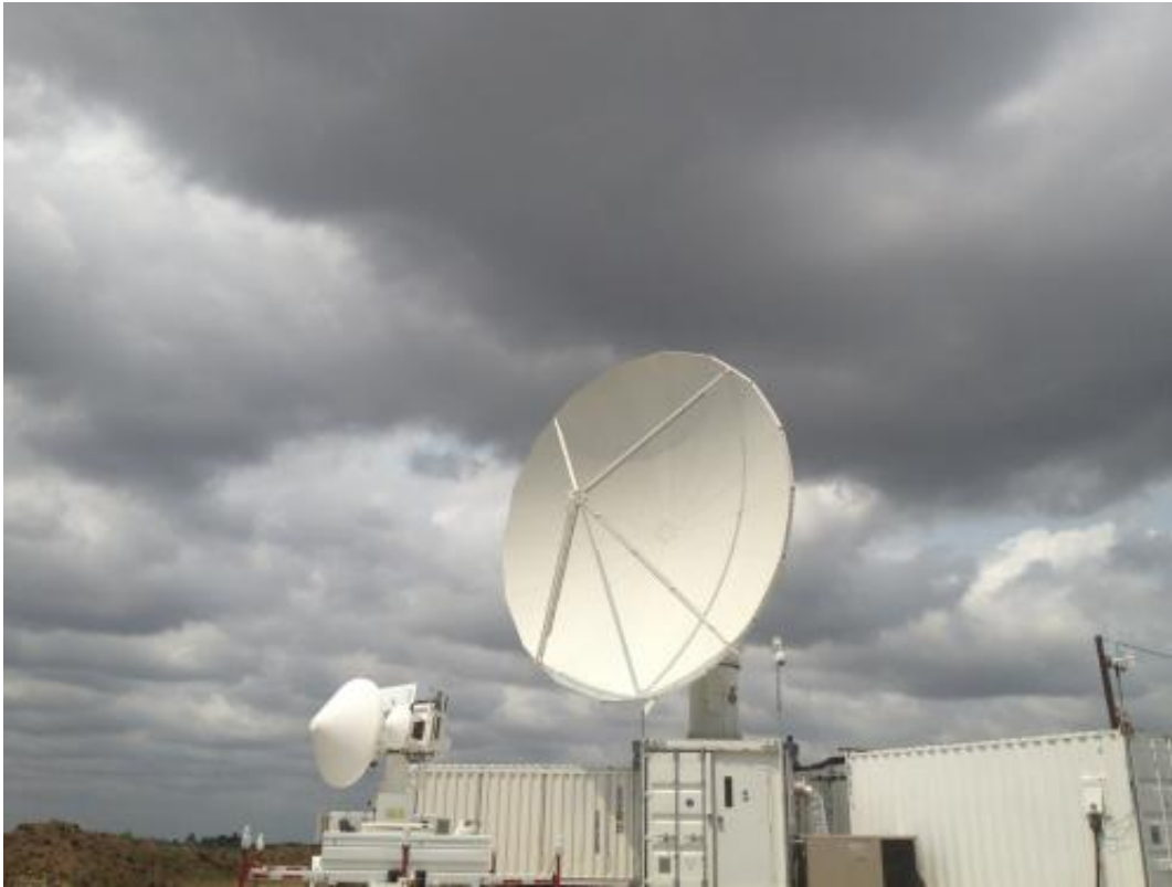
The NASA Polarimetric Radar (right) and Dual-Frequency, Dual-Polarimetric Doppler Radar (left) set up in field near Traer, Iowa. Credit: NASA
