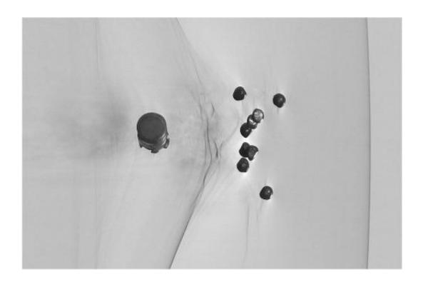
This is a background-subtracted streak image of 00 buckshot, 354 m/s, detail view. Approved for public release: distribution is unlimited. Credit: MetroLaser.
