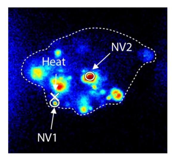
Confocal scan of a single cell. The white cross corresponds to the position of the gold nanoparticle used for heating, while the red and blue circles represent the location of diamond sensors used for thermometry. The dotted white line outlines the cell membrane.
