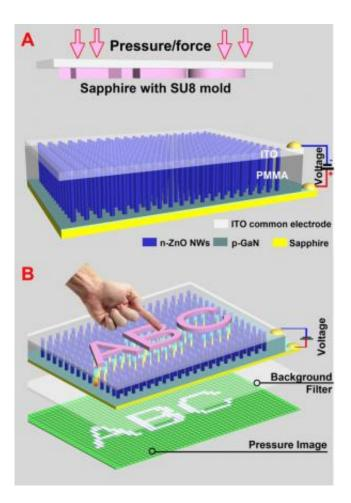
This schematic shows a device for imaging pressure distribution by the piezophototronic effect. The illustration shows a nanowire-LED based pressure sensor array before (a) and after (b) applying a compressive strain. A convex character pattern, such as "ABC," molded on a sapphire substrate, is used to apply the pressure pattern on the top of the indium-tin oxide (ITO) electrode. Credit: Zhong Lin Wang
