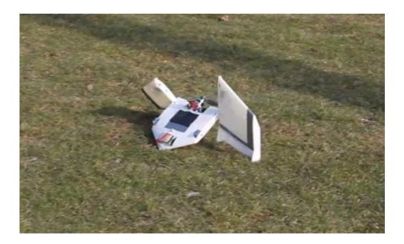
(Phys.org) —At the Laboratory of Intelligent Systems we are developing a novel flying platform which has the ability to move on the ground by using its wings only. Using the wings as whegs to move on rough terrains instead of adding an additional structure to the robot allows to minimize its structural mass.
