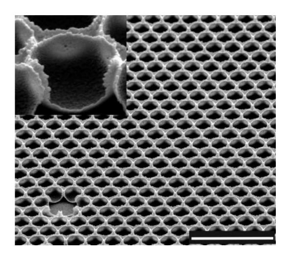
The tiny, tightly packed cells of the honeycomb-like structure, shown here in this electron micrograph, make the SLIPS coating highly durable. Credit: Nicolas Vogel, Wyss Institute
