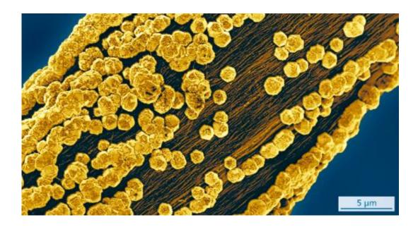
New ultra-thin saw wire for cutting silicon wafers: diamond on top of carbon nanotubes. Credit: Fraunhofer IWM
