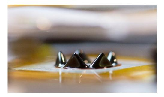
L. Brad King's prototype of a ferrofluid ion thruster. When subjected to voltage, the points of the crown arise from a ring-shaped trench circling a one-inch block of aluminum. Credit: L. Brad King
