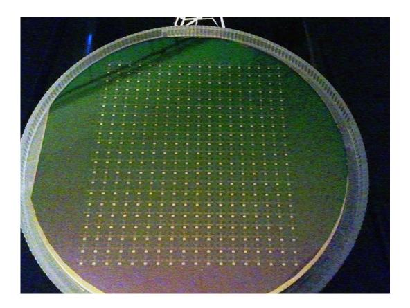
The Miraj Diamond platform resulted from the marriage of two scientific breakthroughs: the ability to deposit nanocrystalline diamond films at relatively low temperatures and a doping process that makes NCD into a good semiconducting material.
