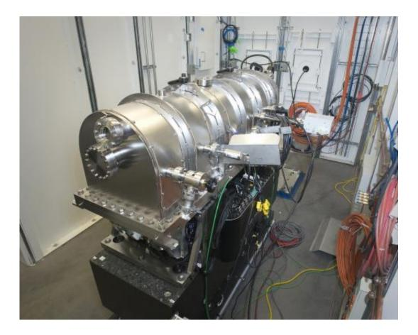
The practically perfect mirror sits within a vacuum chamber mounted on an assembly with springs designed to minimize vibrations.
