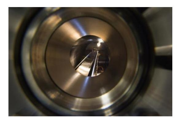
The four-and-a-half foot mirror is pictured here inside its vacuum chamber. The X-ray beam produced at NSLS-II will reflect off the mirror at a very low angle, allowing it to maintain its high energy as it travels toward samples at the end of the beamline.
