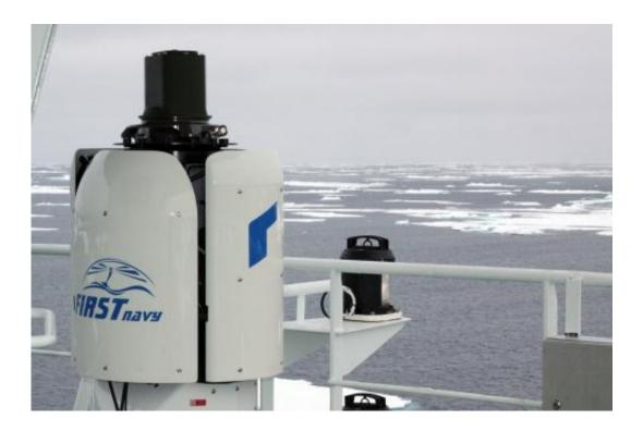
The FIRST Navy thermal imager is installed in Polarstern's crow's nest at a height of about 28 m above water on a highly stabilized platform (white basis). The sensor head (green) rotates at 5 revolutions per second. In the crow's nest the wind often blows at gale force strength due to the ship's superstructure while the temperature plummets to minus 30° C, presenting highest demands to the system. Credit: Lars Kindermann, Alfred Wegener Institute
