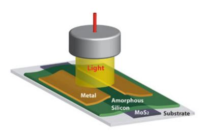
Shown is an experimental photodetector made out of amorphous silicon and molybdenum disulfide (MoS2).
