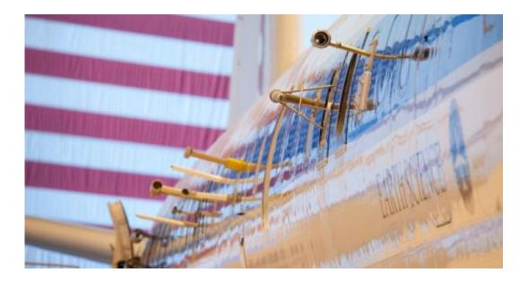
A number of atmospheric probes are installed along the fuselage of NASA's DC-8 in preparation for the SEAC4RS study to learn more about how air pollution and natural emissions affect climate change. Credit: NASA / Tom Tschida
