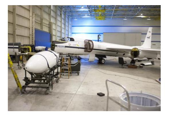
The equipment bays and wing pods of NASA's high-altitude ER-2 will carry 15 specialized instruments to study how the vertical convection of air pollution and natural emissions affect climate change. Credit: NASA / Tom Tschida
