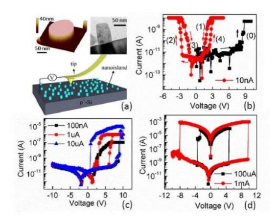
This is a series of images that shows the zinc oxide nano-island on silicon and the three modes of the operation. Credit: University of California, Riverside
