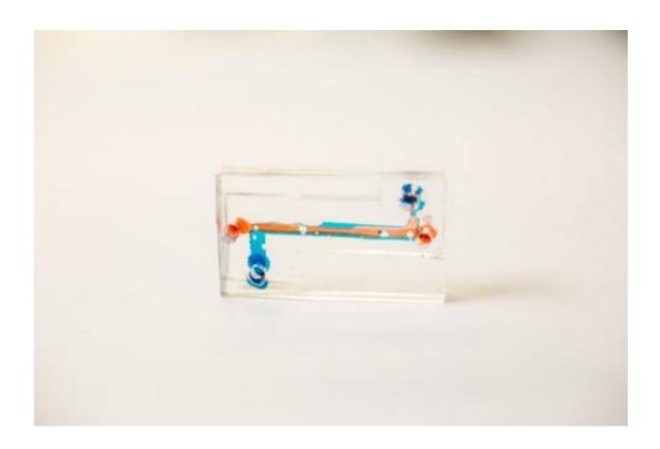
A finger-sized chip will be etched with channels that mimic the branching capillaries of the human lung.
