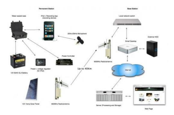
This is a schematic of the components of the ARBIMON recording system. Credit: ARBIMON
