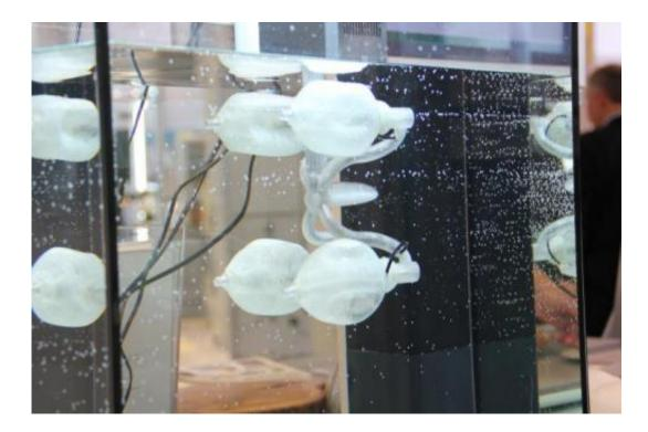
Four elastomer balls pump water and provide the required propulsion. The propulsion system was produced with the fused deposition modeling (FDM) generative production process. Credit: Fraunhofer IPA
