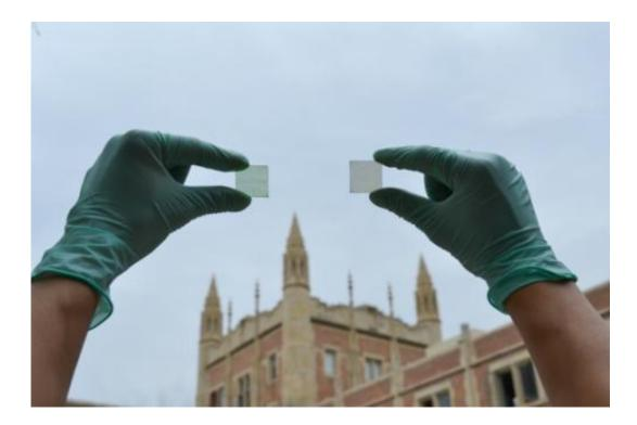
UCLA researchers have developed photovoltaic cells with twice the energy harvesting capacity of cells developed in 2012. The cells, which can be processed to be transparent or in shades ranging from light green to brown, could be used to make building windows, smartphone screens, car sunroofs and other surfaces into sources of sustainable energy.
