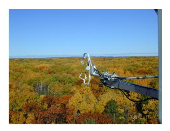
A sonic aenomometer and air inlet tube on an eddy-covariance tower at University of Michigan Biological Station, Michigan, USA. The instruments allow for the continuous monitoring of gas exchange between the forest and the atmosphere. Credit: Chris Vogel
