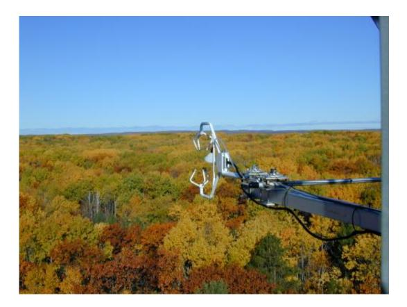
A sonic aenomometer and air inlet tube on an eddy-covariance tower at University of Michigan Biological Station, Michigan, USA. The instruments allow for the continuous monitoring of gas exchange between the forest and the atmosphere. Credit: Chris Vogel
